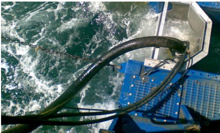
Figure 10 LSS 12m, oil hose connected to weir skimmer module
