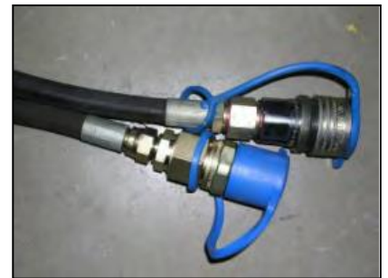
Figure 16 Hydraulic couplings
