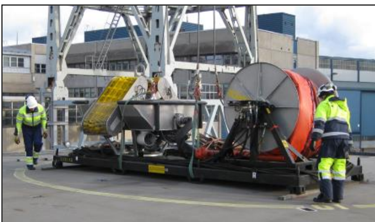
Figure 28 Flat rack container for LAS 125 W/P Skimmer
