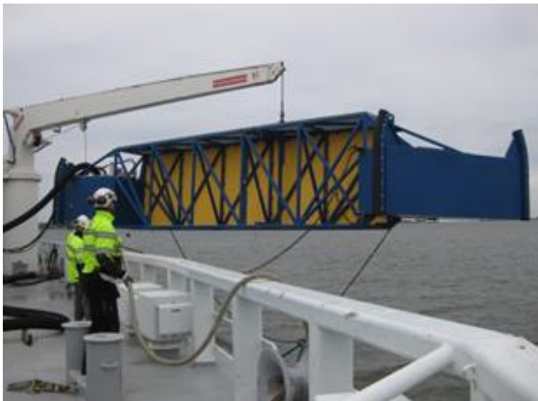
Figure 1 LAMOR Stiff Sweeping Arm system LSS 12m
