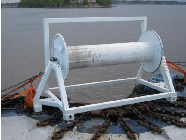
Figure 17 Lamor guiding roll for boom reel
