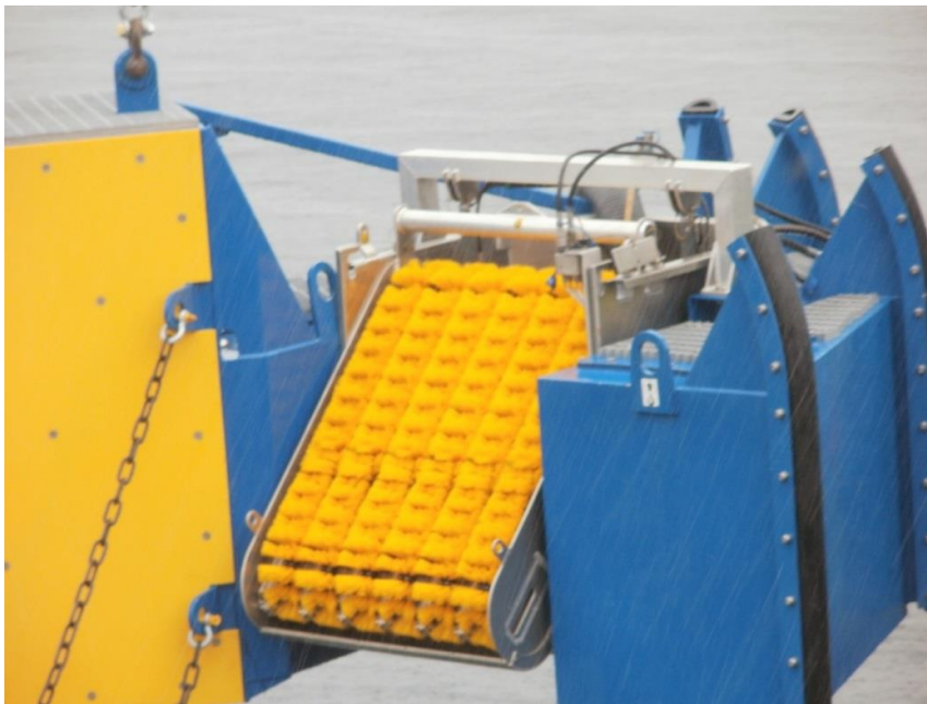
Figure 5 LAMOR Stiff Sweeping Arm LSS 12m – brush skimmer module
