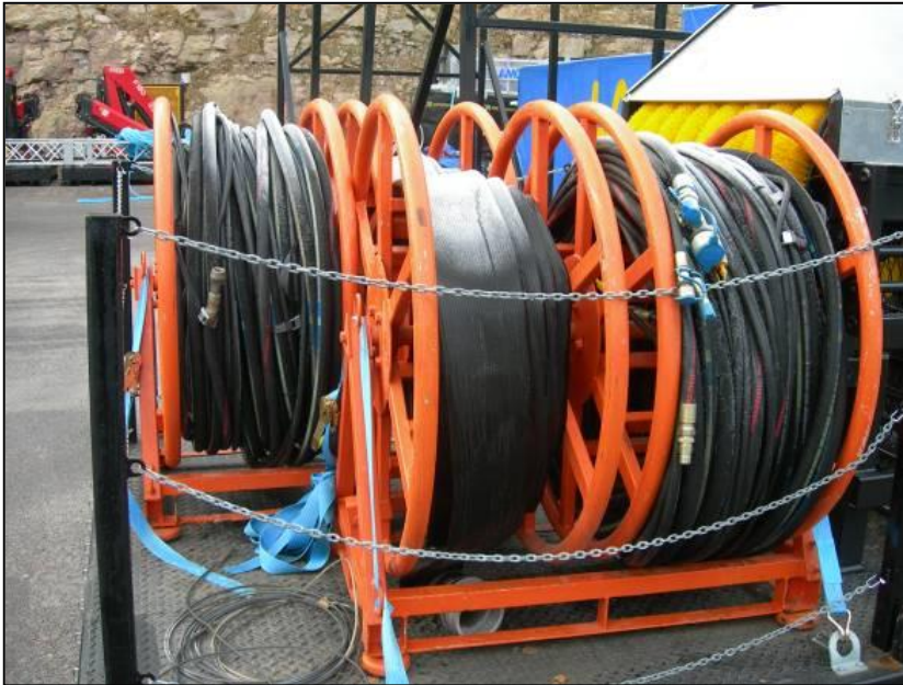
Figure 27 Hose Winder for LAS 125 W/P Skimmer with oil and hydraulic hoses
