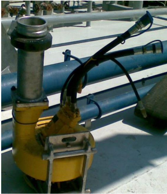
Figure 6 Mariflex Centrifugal Pump MSP150
