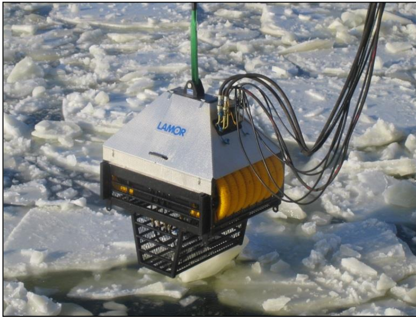
Figure 24 Brush Arctic Skimmer LAS 125 W/P brush module
