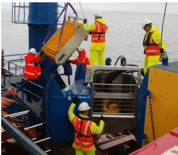
Figure 3 LAMOR Stiff Sweeping Arm LSS 12m – weir skimmer module on the front
